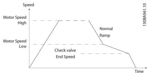
Figure 3.24 Check Valve Ramp
