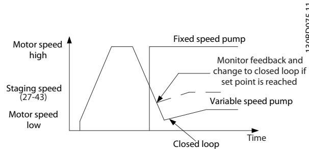
**Figure 3.107 Staging Threshold****27-46 Staging Speed [Hz]****Range:****Function:**
