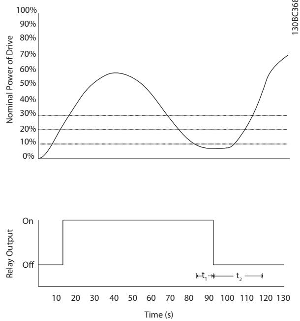
Figure 3.33 Example of the Output Function
