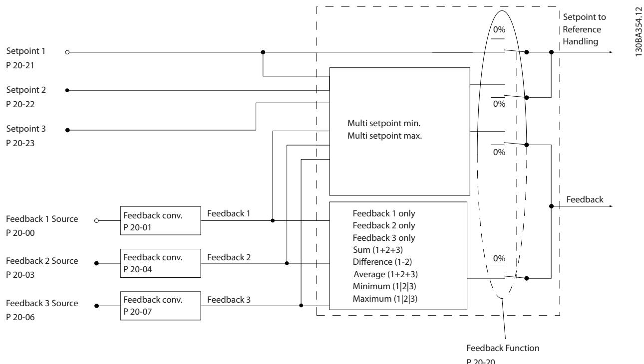
Figure 3.60 Input Signals in Closed-loop PID Controller
