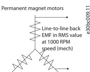
Figure 3.7 Machine Parameter Definitions of Back EMF of PM Motors
