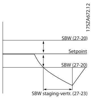
Figure 3.100 SBW Staging Delay
