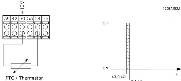
**Figure 3.14 PTC Thermistor Connection - Analog Input**
