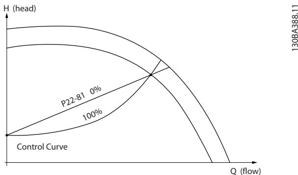
Figure 3.71 Square-Linear Curve Approximation
