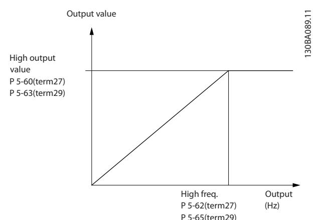
**Figure 3.32 Pulse Output**
