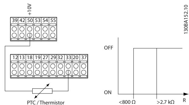
Figure 3.13 PTC Thermistor Connection - Digital Input
