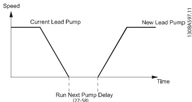
Figure 3.109 Run Next Pump Delay
