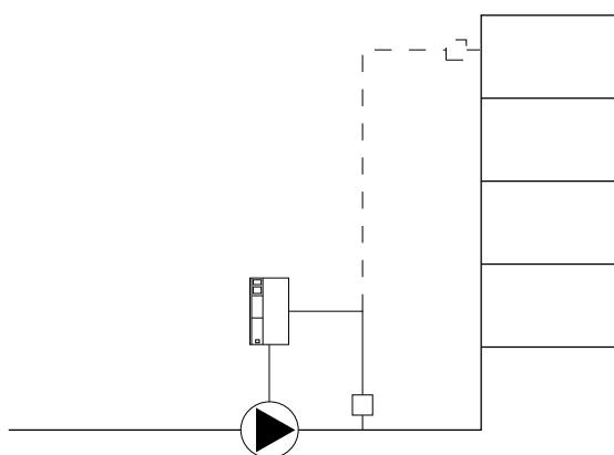
Figure 3.70 Flow Compensation Set-up
