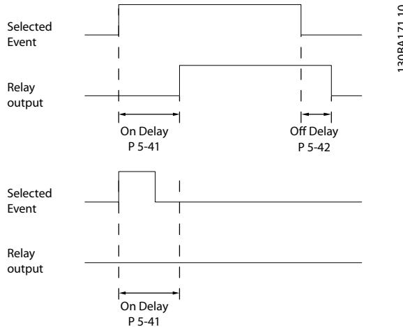
Figure 3.29 On Delay, Relay
