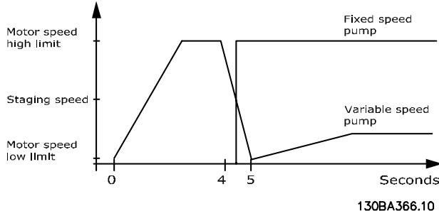
Figure 3.90 Staging Threshold
