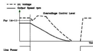
**Figure 3.51 Controlled Ramp Down, Longer Mains Failure.**
