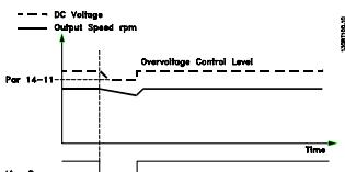
Figure 3.52 Kinetic Back-up, Short Mains Failure
