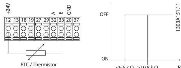
Figure 3.16 Thermistor Connection
