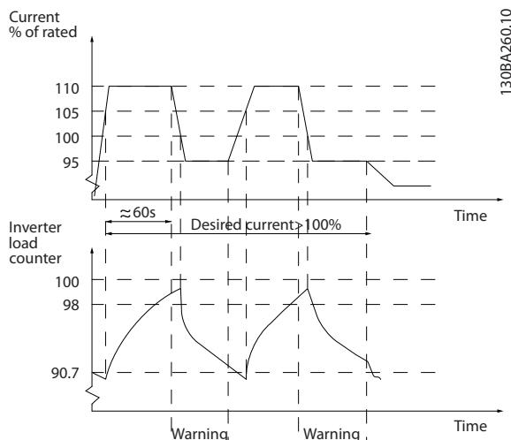
Figure 3.55 Output Current in Overload Condition
