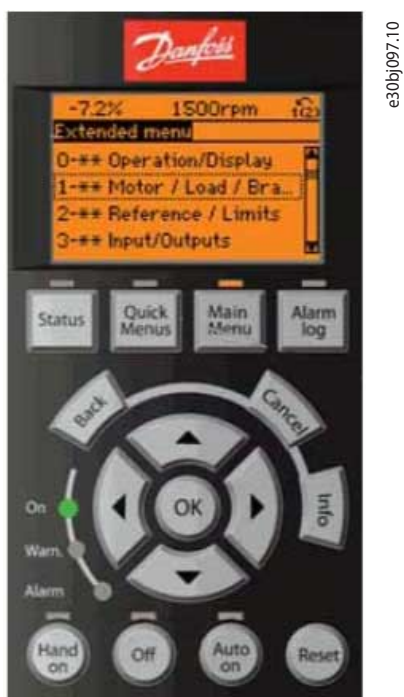
Illustration 22: Graphical LCP Display (Order Code 132B1107)
