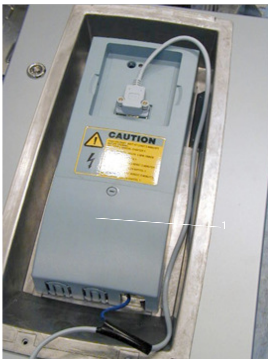
Illustration 4: Attach the cable cover after connecting the grounding cable, FR8
