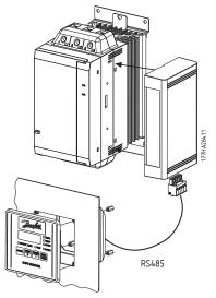
Remove mains and control voltage from the soft starter before attaching or removing accessories. Failure to do so may damage the equipment.
