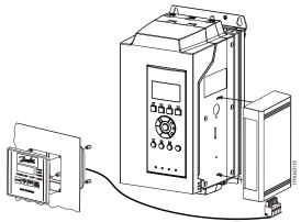
Remove mains and control voltage from the soft starter before attaching or removing accessories. Failure to do so may damage the equipment.
