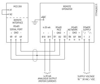
For the Remote Operator to accept serial commands, a link must be fitted across terminals A1-N2 on MCD 200 starters.
