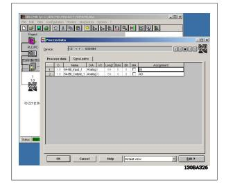
When the system is running, change the state to: *Monitor*. Click on the controller board and select: Address Monitor.
