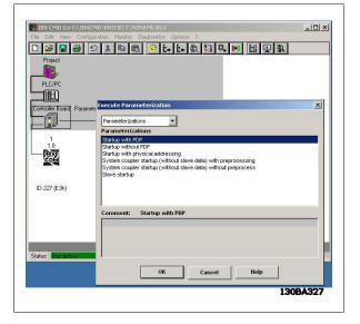
The state will be changed from Offline to Online when the Read In is finished. Please look at the bottom of the screen. After the Read In, CMD will indicate each VLT frequency converter with a DriveCom symbol, a station number and an ID number.
