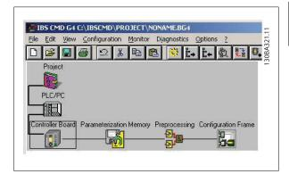
The next step is to read the slaves into the bus system. Click on Configuration frame and click on the right mouse button. Select Read In (from memory).
