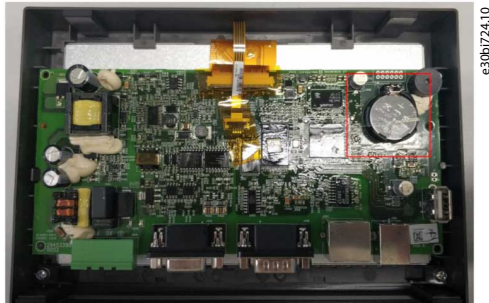
Illustration 75: Location of the Battery Inside the HMI
