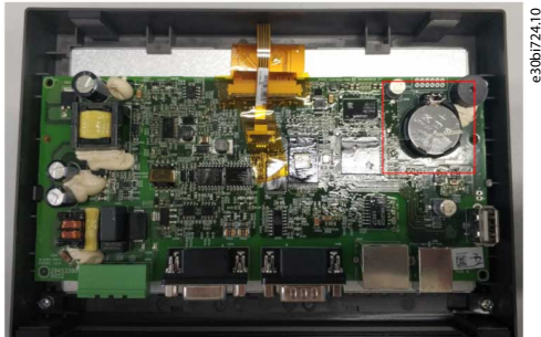
Illustration 75: Location of the Battery Inside the HMI
