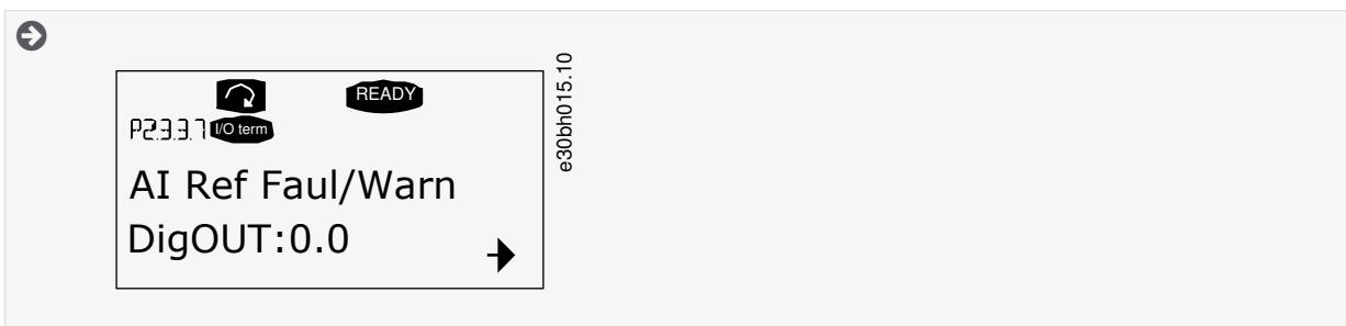
2. When the value is blinking, hold down the Browser button up or down to find the desired board slot and signal number. The program scrolls the board slots starting from 0 and proceeding from A to E and the I/O selection 1–10.
