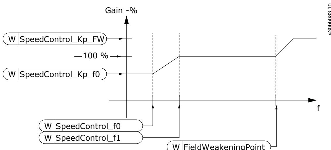
Illustration 101: Speed Controller Adaptive Gain
