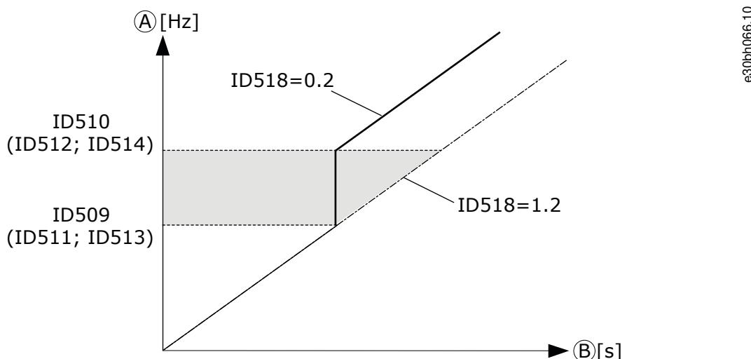
**Illustration 72: Ramp Speed Scaling between Prohibit Frequencies**
