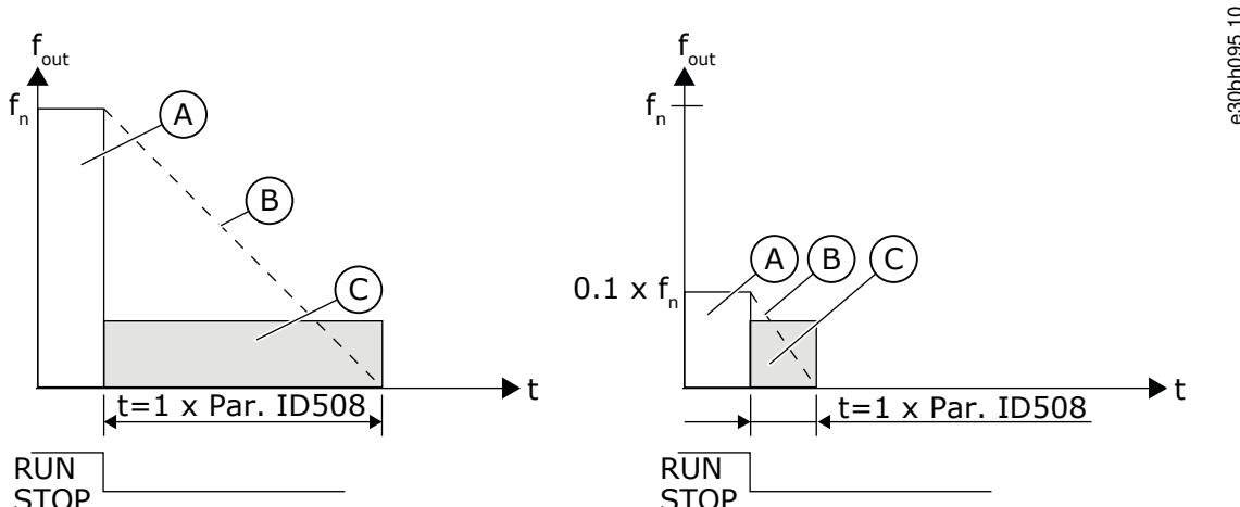
Illustration 69: DC-Braking Time when Stop Mode = Coasting
