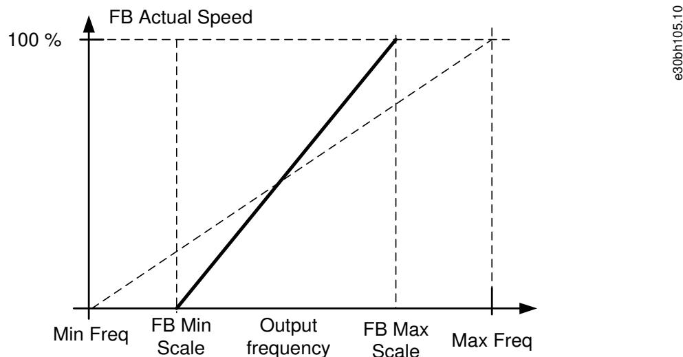
**Illustration 81: Fieldbus Minimum and Maximum Scaling Effect on Actual Value**
