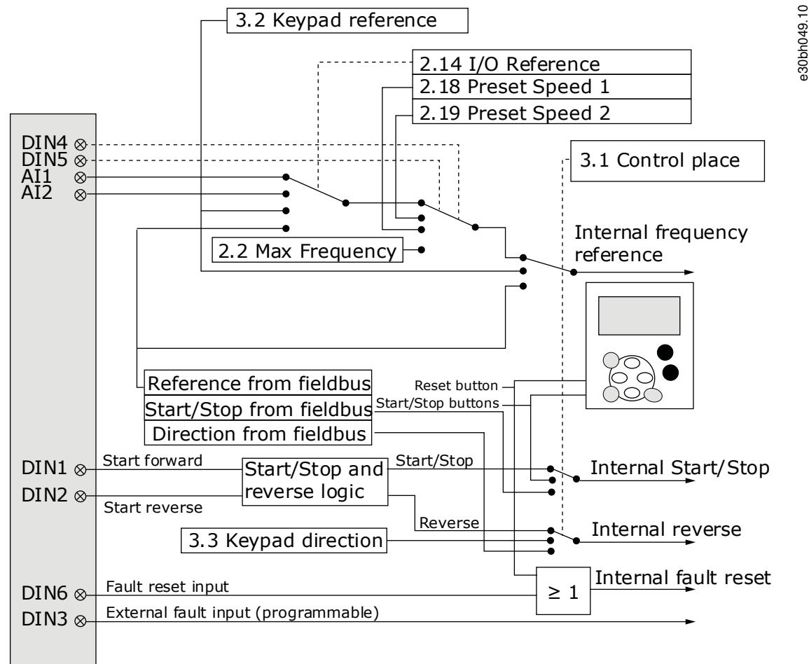
Illustration 4: Control Signal Logic of the Basic Application
