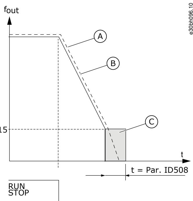
Illustration 70: DC-Braking Time when Stop Mode = Ramp
