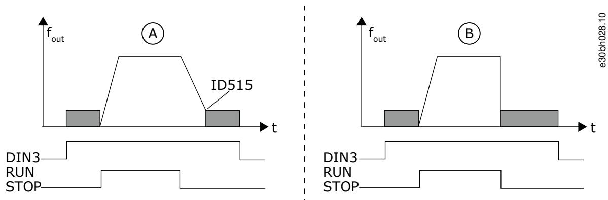
**Illustration 34: DIN 3 as DC brake Command Input**
