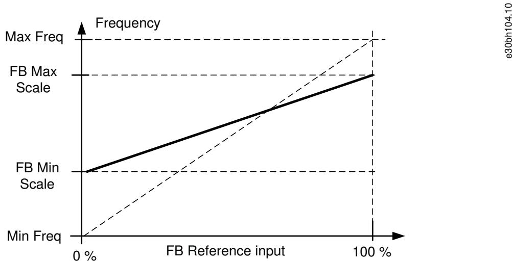
**Illustration 80: Fieldbus Reference Minimum = Maximum Scaling**
