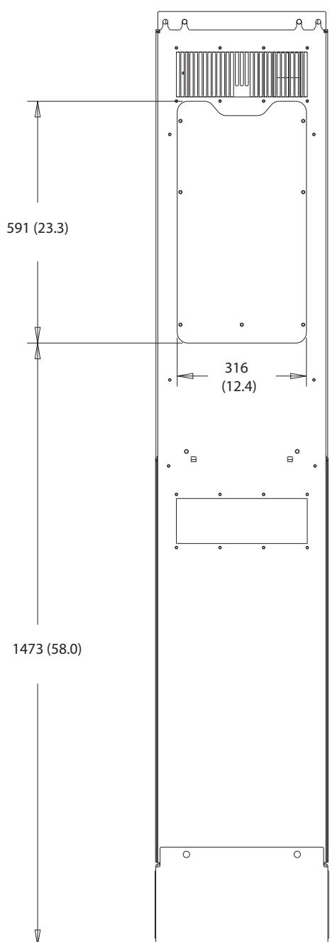
Illustration 10.40 Heat Sink Access Dimensions for D8h
