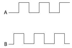
**Illustration 8.6 Determining Encoder Direction**
