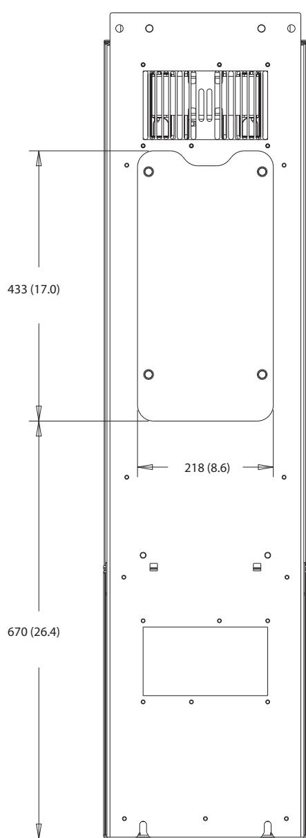
**10****Illustration 10.21 Heat Sink Access Dimensions for D5h**
