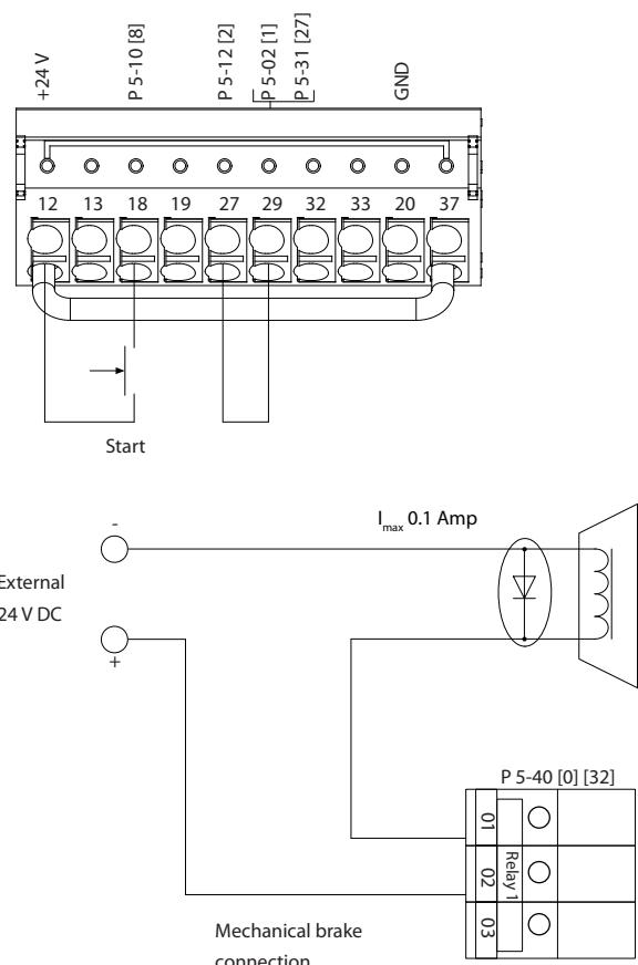
**Illustration 8.8** Wire Configuration for Torque and Stop Limit
