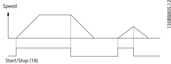
Illustration 8.2 Start/Stop with Safe Torque Off
