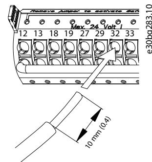
Illustration 5.37 Connecting Solid Control Wires
