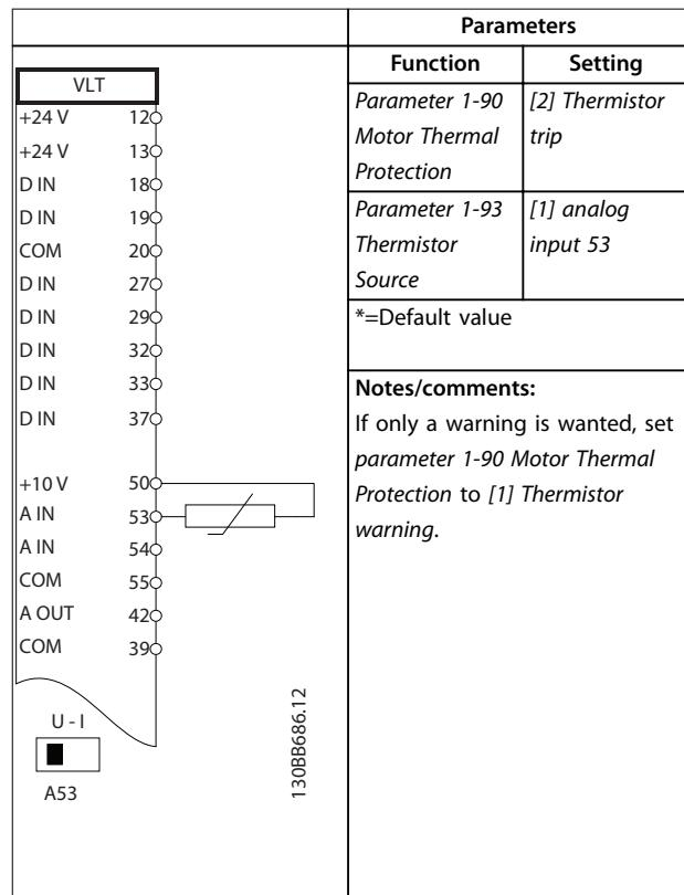
**Table 8.12 Wiring Configuration for a Motor Thermistor**
