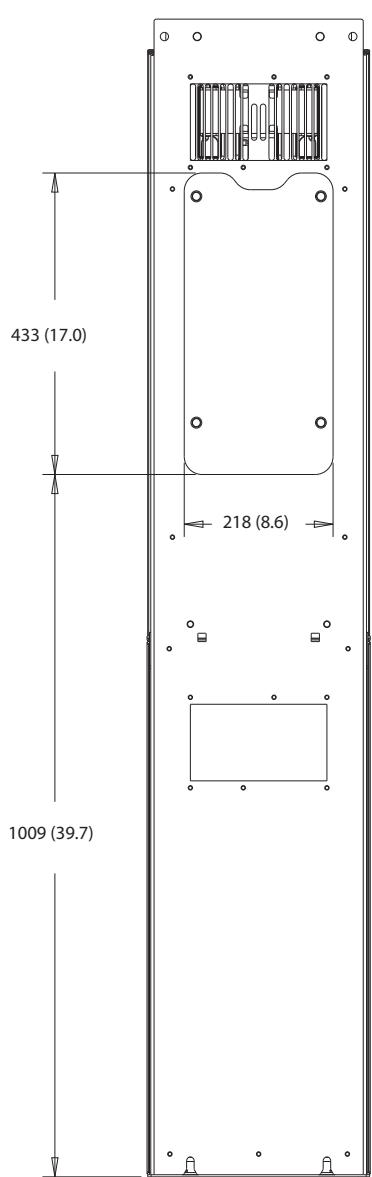
Illustration 10.27 Heat Sink Access Dimensions for D6h
