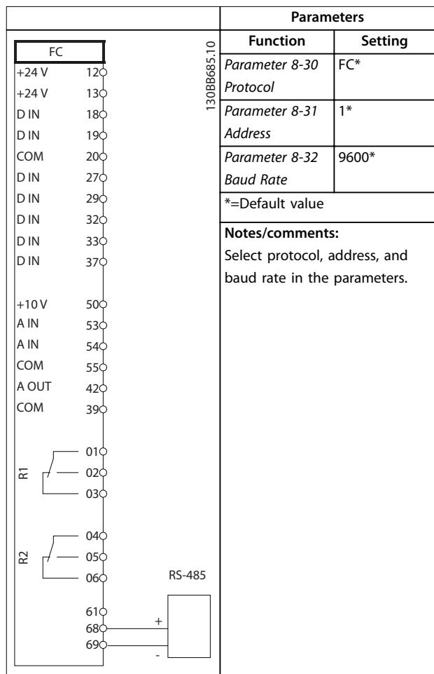
**Table 8.11 Wiring Configuration for RS485 Network Connection**
