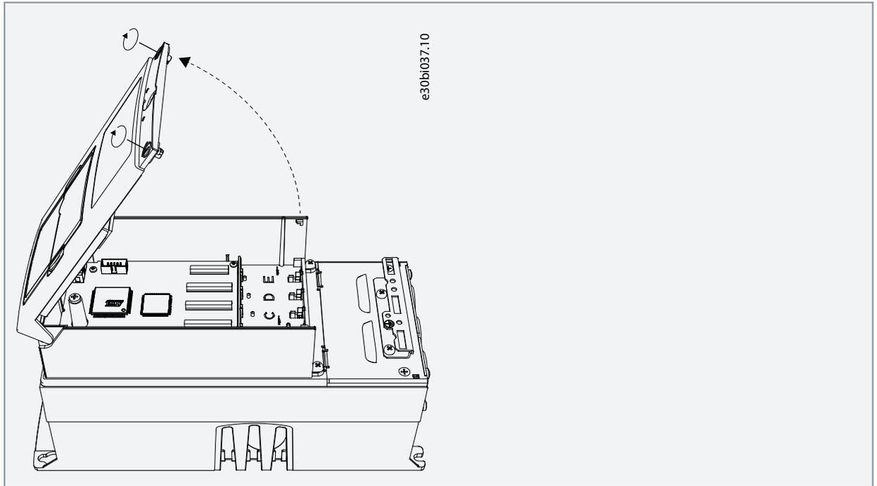
4. Install the option board into the slot C, D, or E on the control board of the AC drive. Make sure that the grounding plate fits tightly in the clamp.
