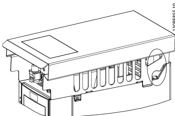
Illustration 1.5 Frequency Converter with IP21/Type 1 Conversion Kit
