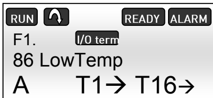
Figure 7.1-3, Low temperature alarm on the NXP panel
