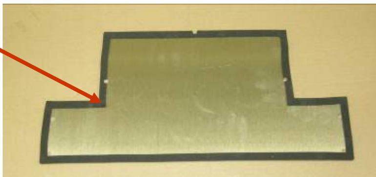
Install the top duct cover plate as shown using the new 16mm, M5 screws provided with the kit
