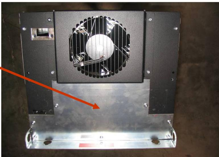
Install the two mounting clips on the bottom of the frame as shown. Note that the E2 frame VLT utilizes six mounting clips for the bottom cover plate.
