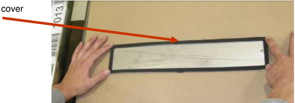
Install the bottom cover plate as shown.
