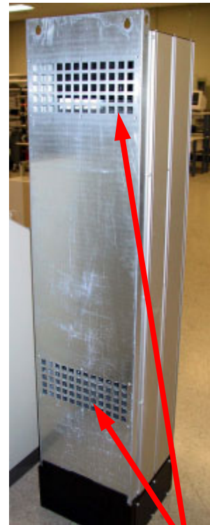
Photo 1. Drive openings on rear are not used in this application.
