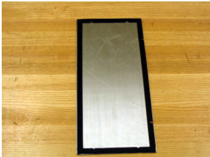
Photo 16. Top duct closing plate with gasket.
