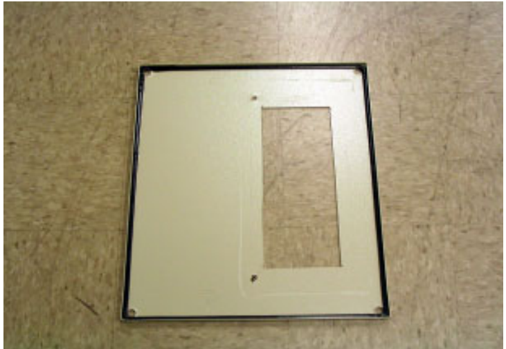
Photo 9. Enclosure top with cutout.
