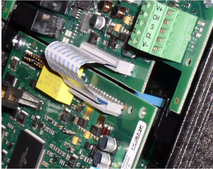
Figure 4: Flexible Circuit Interface to Control Board
