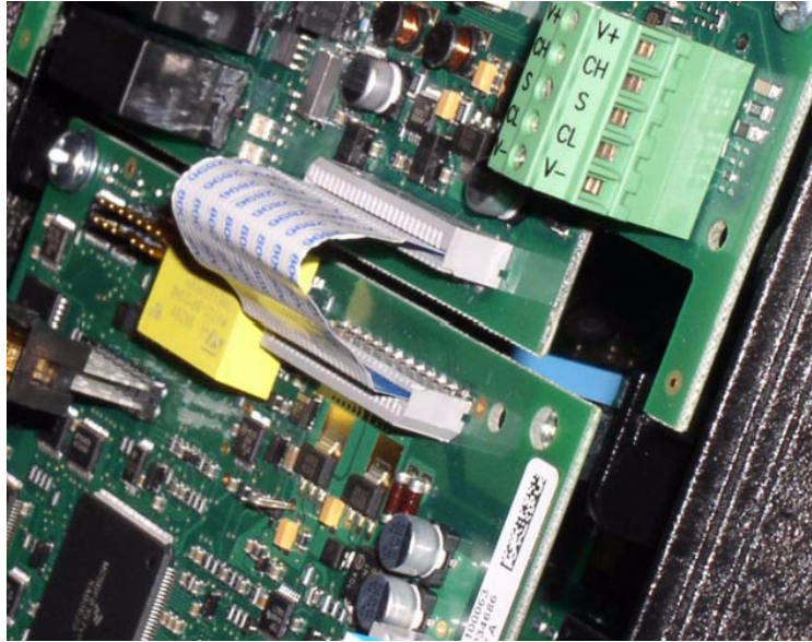
Figure 4: Flexible circuit interface to control board
