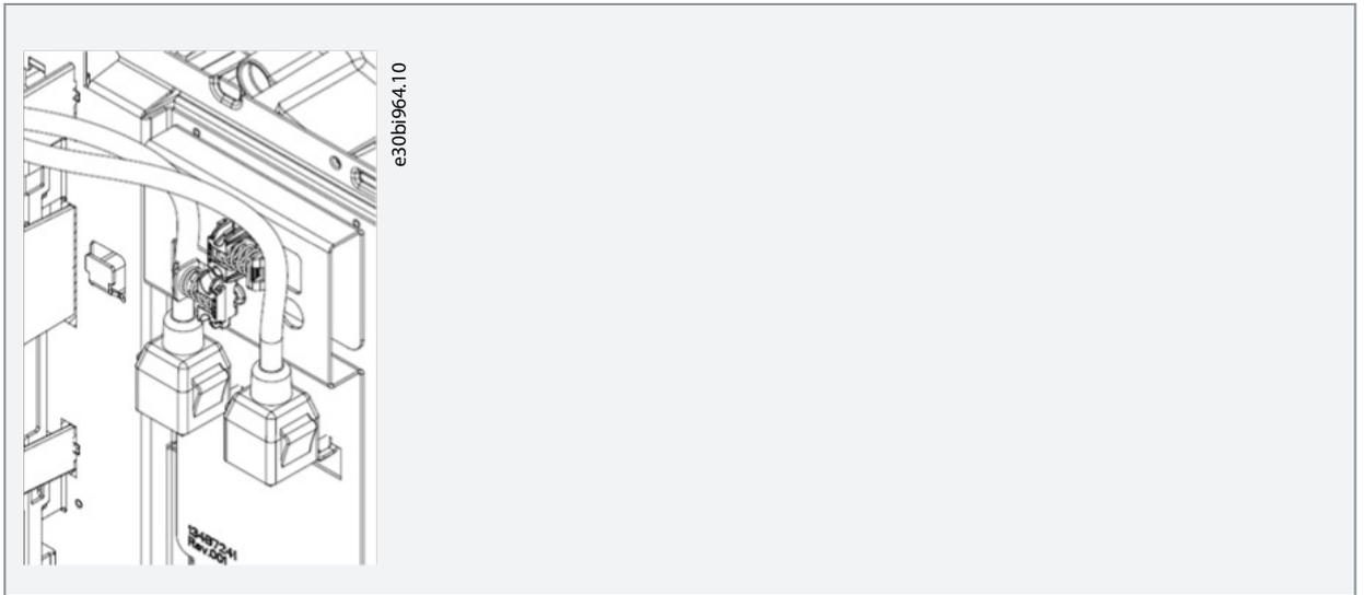
8. Connect the external Ethernet cable to the internal extensions cables on the option.
