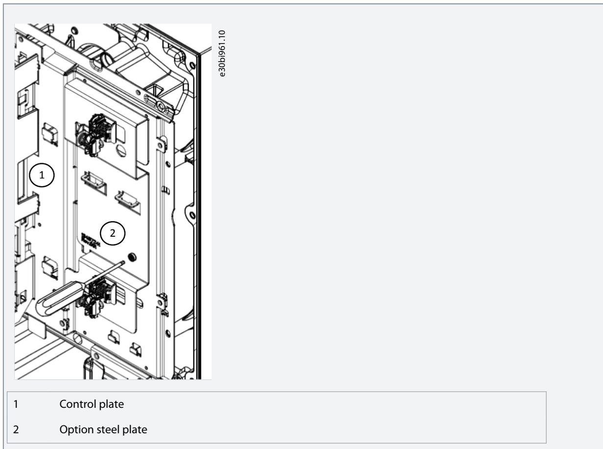
5. Tighten the 2 T10 screws to 1.2 Nm (10.62 in-lb)
