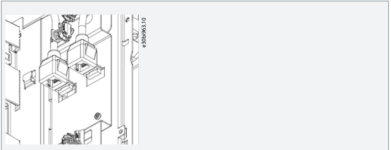
7. Connect the Ethernet cables to the Ethernet option card and click the cables into the cable hooks.
