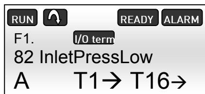
Figure 7.1-4, Low pressure alarm on the NXP panel
