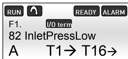
Figure 7.1-4, Low pressure alarm on the NXP panel
