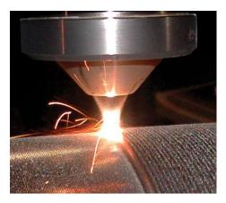
Hydroclad™ laser cladding was the first anti-corrosion coating technology to earn JIP Certification - DNV's guideline for qualification of wear and corrosion protection of surface materials for piston rods.
