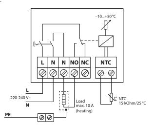
IMPORTANT: When the thermostat is used to control a floor heating element in connection with a wooden floor or similar material, always use a floor sensor and never set the maximum floor temperature to more than 35°C.
