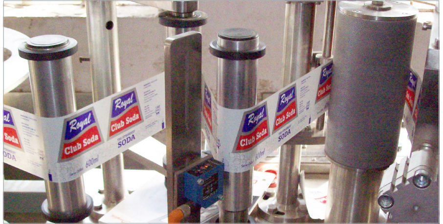
On the cutter roller a zero mark sensor is mounted, and on the feed roller a print marker sensor.
