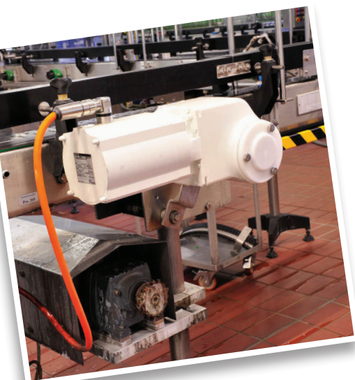
Close-up view of VLT® OneGearDrive® and the old motor solution it replaced before it was unmounted
