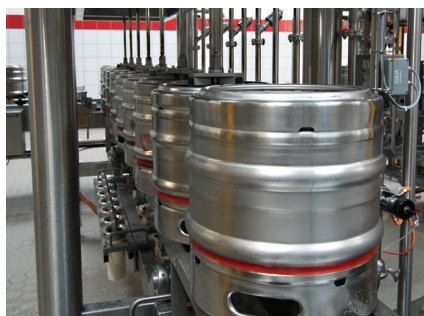
Modernisation of the plant also boosted filling capacity from approximately 120 kegs per hour to as much as 280. The filling line is fully automated; the only task that requires manual effort is supplying pallet stacks with 6 kegs on each pallet to the infeed using a stacker
