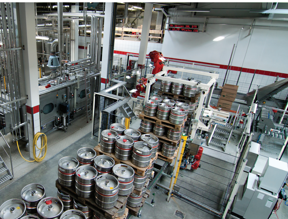
In early 2011 a new, fully automated keg filling line that handles everything from cleaning to palletising was put into service. It is optimally integrated in the overall structure and reduces path lengths
