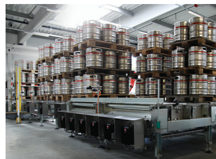
Pallet transport motors in the dry area are controlled by 40 VLT® Decentral Drive FCD 300 units. They are fitted with covers for protection against falling kegs
