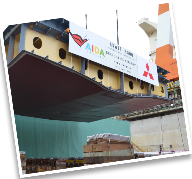
The first keel element for AIDA's luxury cruise ship is lowered into place at Mitsubishi Heavy Industries Shipyard, Japan
