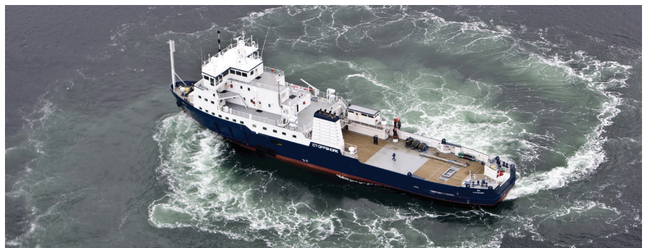
The new dynamic positioning system with electric tunnel thrusters is able to hold the SIA in position with a precision of 200 mm.
