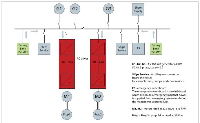
Example of Power Limit function running on board a hybrid ship. If one generator trips, power is limited to the other two generators to ensure they are not overloaded, and can continue running.
