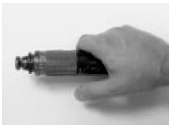
Figure 1 - Holding the Insertion Tool
