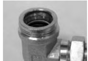
Figure 5 – Properly Assembled O-ring & B-ring
