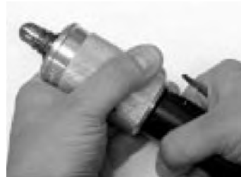
Figure 3 – Twisting Tool To Release
