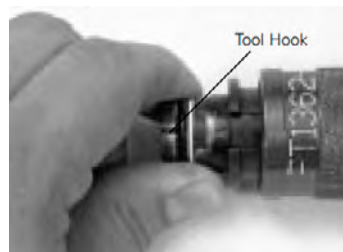
Figure 2 - Squeezing the O-ring & Backup Ring
