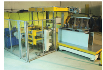
The press table has four independent servo hydraulic axes positioned around the side and front walls which allows the upper table to be positioned parallel to the product table
