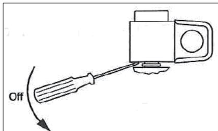
Remove the clip-on coil by using a screw driver.
