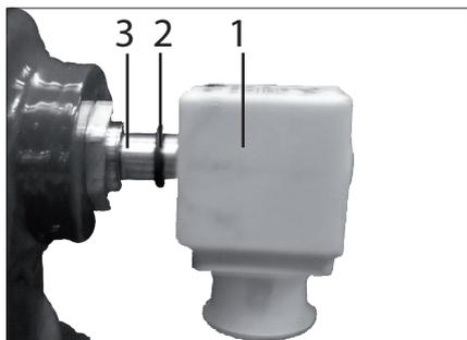
Put the clip-on coil (1) with the gasket (2) over the valve body (3) on the compressor
