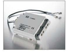
The time delay relay type SD is designed for staggered start of two compressors in the Twinversion as the one-phase mains cannot normally be loaded with the total starting current of both compressors.
