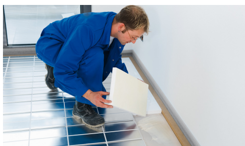
Fig. 5: Light constructions (e.g. laminate/engineered timber or strongboard constructions laid directly on the heat panels): rooms > 12 m 2 glue all perimeter and header panels, rooms < 12 m 2 glue all panels (recommended).
