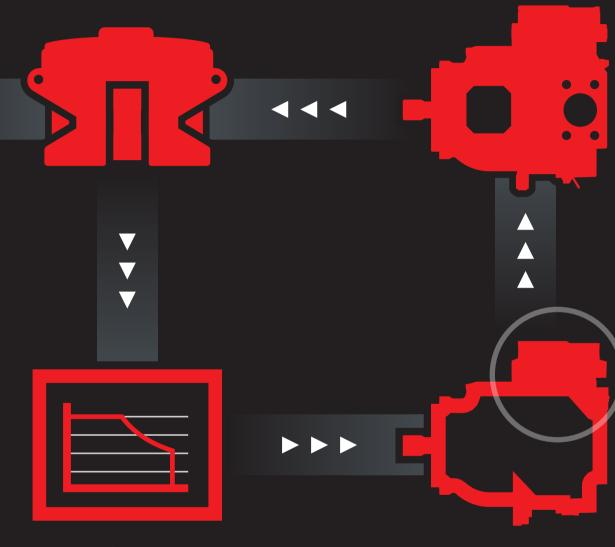
PLUS+1 GUIDE software adjusts the pump's proportional relief valve (PRV) setting for each respective displacement at a given engine speed. GUIDE software blocks are available — allowing for easy integration into existing GUIDE software applications.
