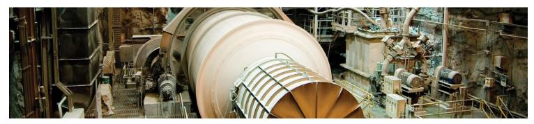
The Airflex® High Energy Ventilated Constricting Clutch expands the energy capacity of traditional drum-clutch products and is designed to sustain high torque at high temperatures.
