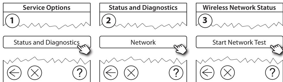
At the end of the network test the Danfoss Link™ CC awaits for all battery operated devices to wake up and report. Follow the instructions given on the screen. If the network test is running smoothly, there will be no need for further interaction. If the network test is performing slow, the Danfoss Link™ CC guides through troubleshooting and gives useful tips for speeding up the process.
