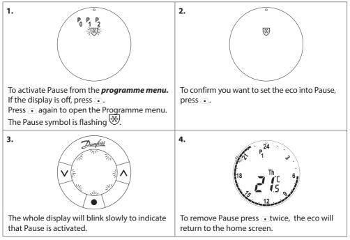
Note! The default Pause temperature is 6  $^{\circ}$ C, to adjust the Pause temperature see chapter 4.9.
