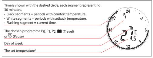
\* eco is displaying the set temperature, not the measured room temperature.
