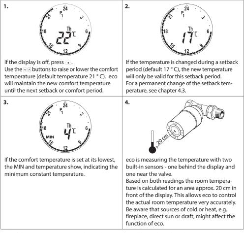
Note! If the set temperature is raised more than 1 °C eco will boost the radiator heat to reach the new temperature faster. You can feel the valve and radiator are getting warmer. Minor temperature changes will not evoke a heat boost, and so the changes are made without any immediate indication.
