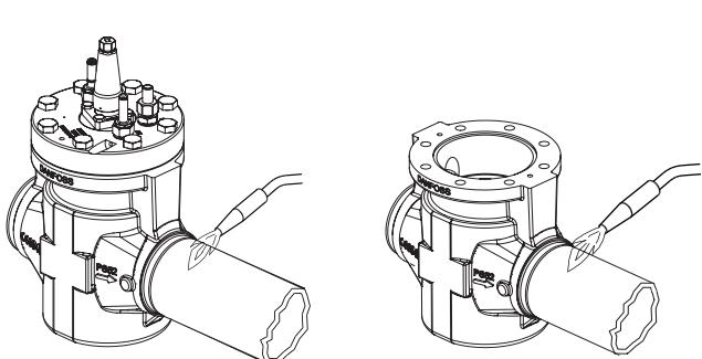
Only for heat controlled welding with no welding debris.
