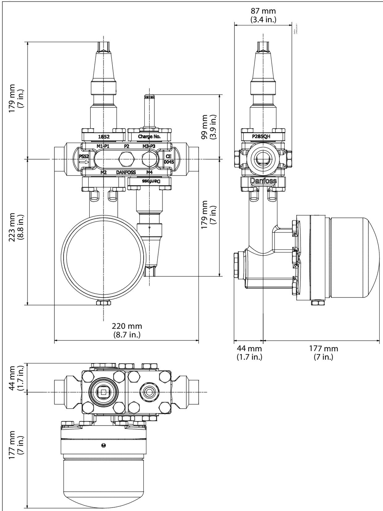
**NOTE:** This example indicates the maximum dimensions for the ICF valve stations.
