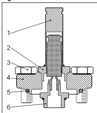
Table 41: ICFA 20 electronic expansion valve module
