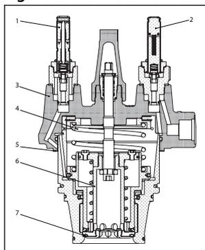
Table 65: ICLX 50 / ICLX 65 2-step solenoid valve module
