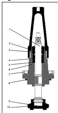
Table 60: SVA-S 50 / SVA-S 65 shut-off valve module
