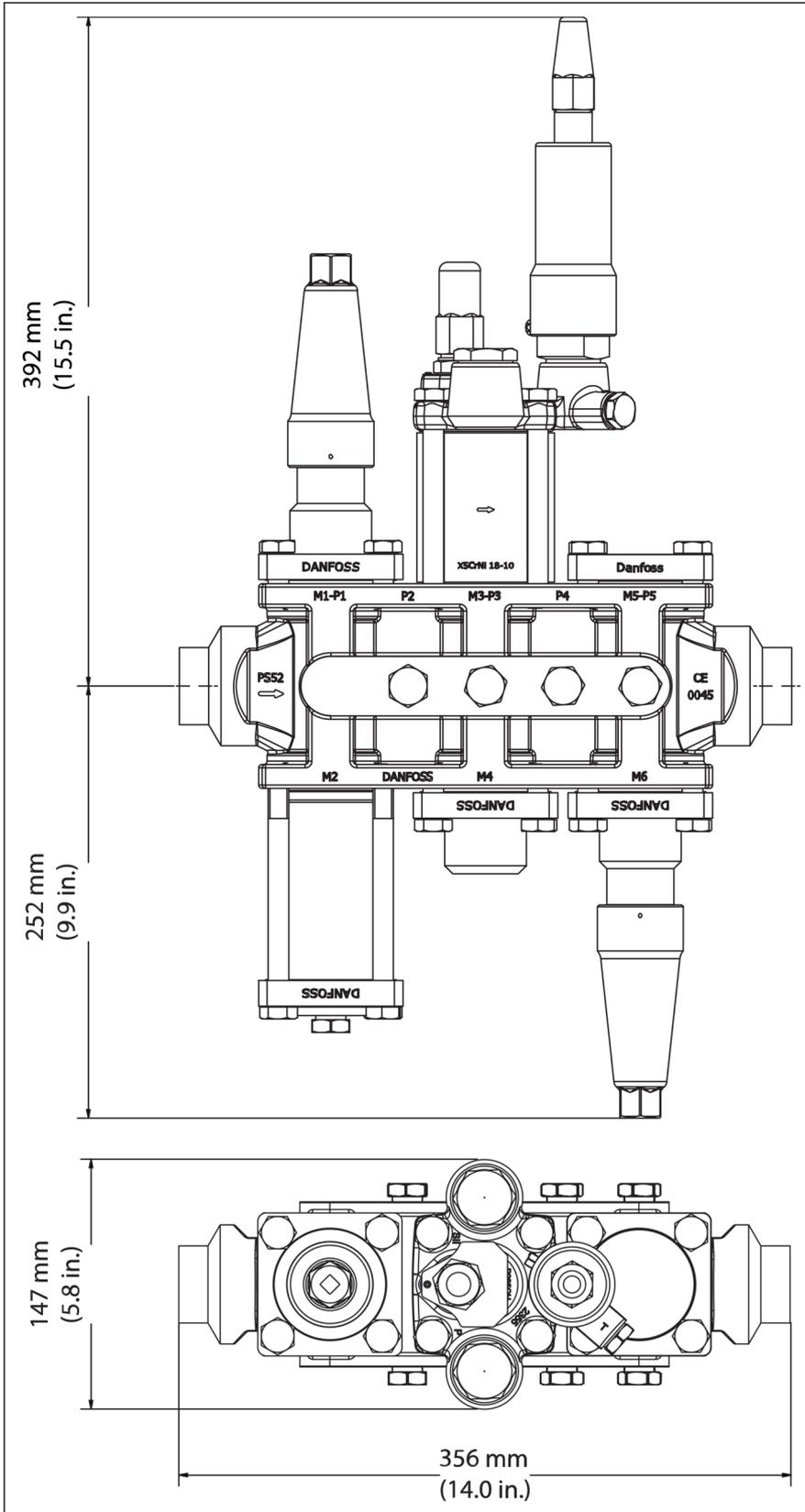
**NOTE:** This example indicates the maximum dimensions for the ICF valve stations.
