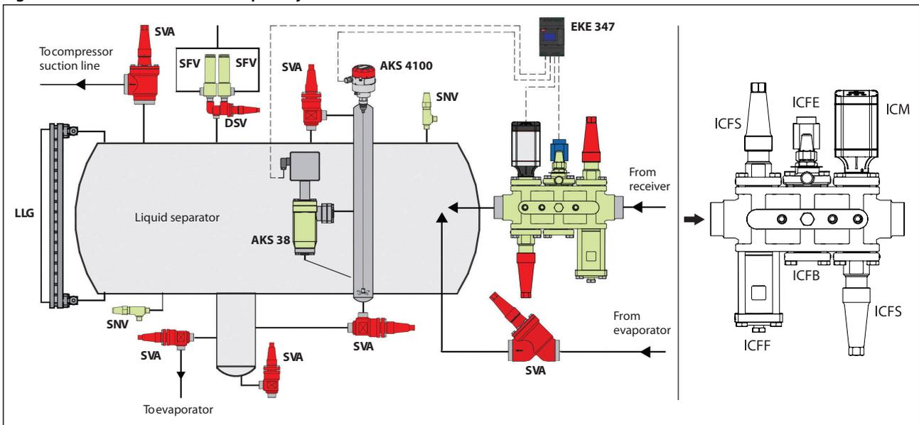
A valve combination for compressor liquid injection with electronic injection valve is required. It is required to have a solenoid valve in front of the control valve.
