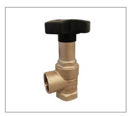
HPBV is a self-acting high pressure bypass valve primarily for use in air-conditioning systems. The controller is normally closed and opens on rising pressure.
