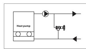
Heat pump system with constant flow circulation pump - HPBV ensures minimum circulation flow through heat pump when system consumption is low and pressure after pump starts to rise.
