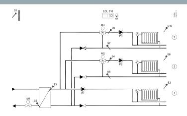
Subtypes A390.3, A390.11, A390.12 and A390.13 have for the control valve 3-point outputs as well as 0 – 10 V outputs
