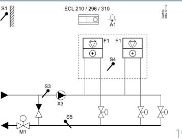
Multi purpose application. Temperature control of, for example, ventilation systems with heating or cooling or a combination of these. Weather based compensation, return temperature limitation, frost and fire protection. Optional analog control of cross-flow or rotary heat exchanger.
