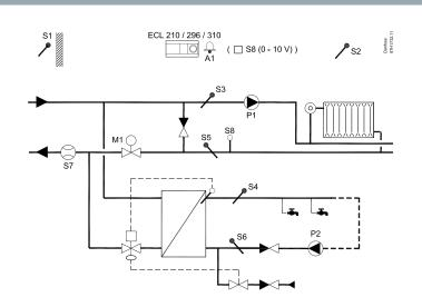
Weather compensated control of flow temperature in a heating circuit. Sliding return temperature limitation. Control of one or two circulation pumps. Optional control of flow temperature related to supply temperature. Refill water function.
