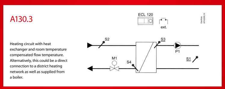
Flow temperature based on compensated supply temperature (offset).
