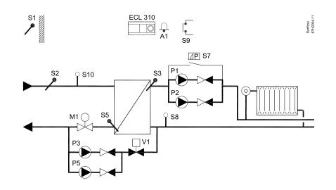
Weather compensated flow temperature control of heating / cooling circuit(s). Automatic change-over between heating and cooling. Circulation pump control. Dew point (cooling mode only) and surface temperature compensation. Return temperature limitation.
