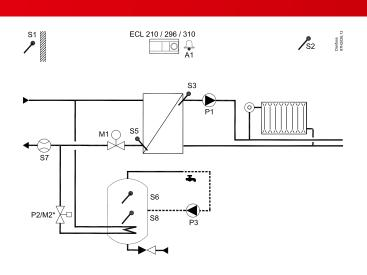
Weather compensated control of flow temperature in heating circuit. Room temperature compensation and sliding return temperature limitation.
