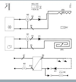
Weather compensated flow temperature control of heating / cooling circuit(s). Automatic change-over between heating and cooling. Circulation pump control. Dew point (cooling mode only) and surface temperature compensation. Return temperature limitation.
