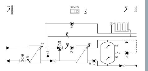
Weather compensated control of flow temperature in heating circuit. Room temperature compensation and sliding return temperature limitation.
