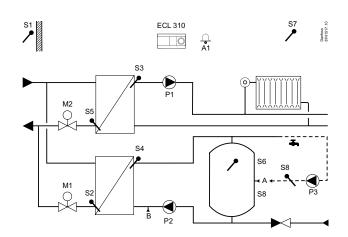
Weather compensated control of flow temperature in two heating circuits. Room temperature compensation and sliding return temperature limitation. Circuits independent in parallel or circuit 2 after circuit 1. Alarm function related to flow temperatures.
