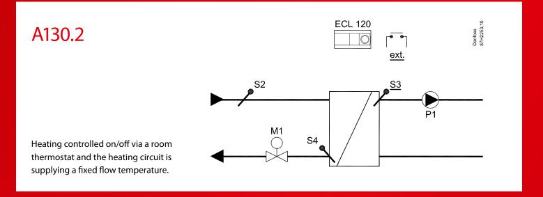
Flow temperature compensated on room sensor.
