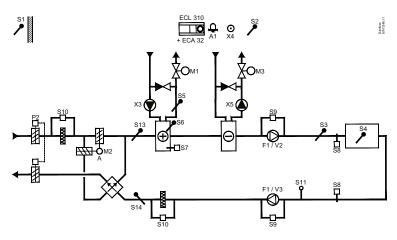
Multi purpose application. Temperature control of, for example, ventilation systems with heating or cooling or a combination of these. Weather based compensation, return temperature limitation, frost and fire protection. Optional analog control of cross-flow or rotary heat exchanger.
