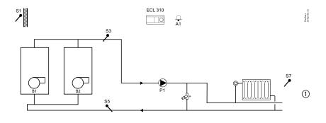
Weather compensated flow temperature control of 1-stage boiler based heating systems. One direct heating circuit and one mixing circuit. Circulation pumps control, room temperature control and sliding return temperature limitation.
