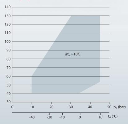
Max. permissible operating pressure (LP/HP) 100/150 bar Compressor version S – compressor ranges HGX12  $\rm CO_2$  and HGX24  $\rm CO_2 T$
