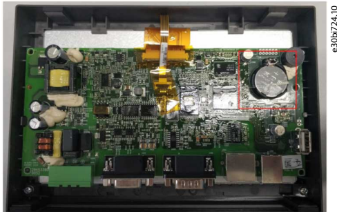
Illustration 87: Location of the Battery Inside the HMI
