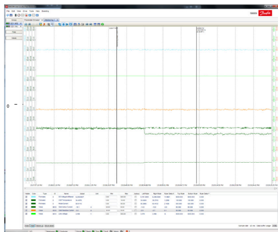
Illustration 89: Monitoring Grid Active Current while adjusting Ref Frame Adapt Angle
