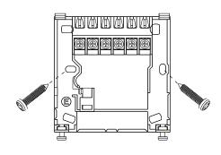
2. Connect the "N" and "L" terminals to the mains power and wire as required for application.
