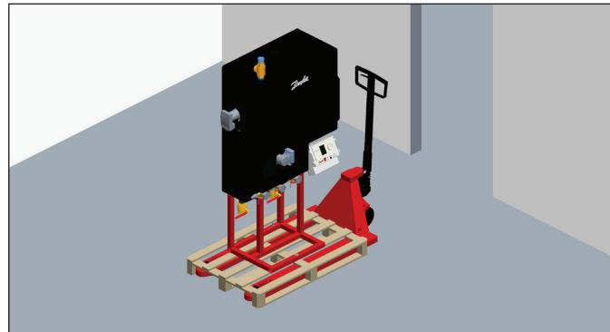
Then detach the system from the pallet; this is fixed using 2 wooden screws.
