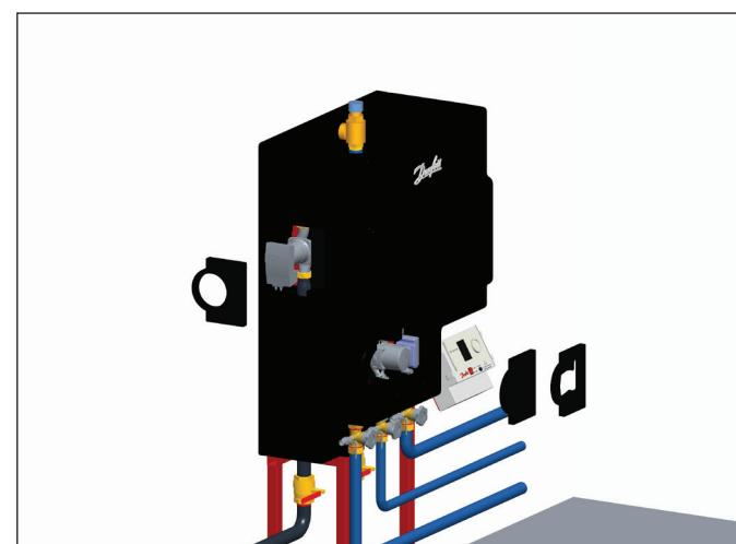
The front cover can be pulled out to the front. This is connected with the rear via multiple connectors (tongue and groove). Pull the cover as far forward horizontally as possible to avoid damaging the connections.
