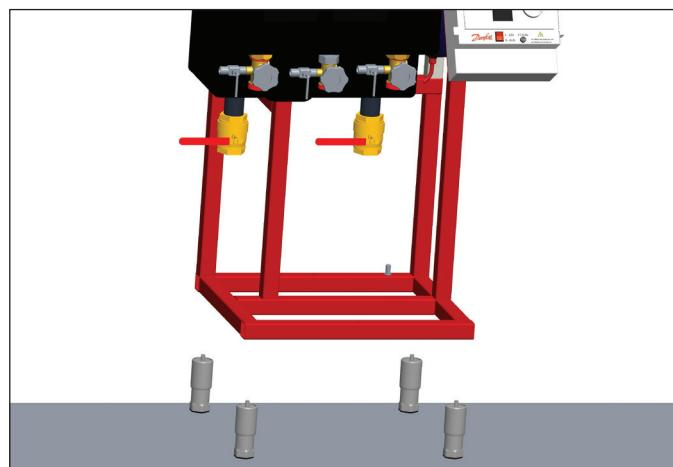
Align the system horizontally by adjusting the height of the feet, e.g. using a spirit level.
