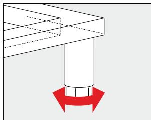
For more uneven surfaces, it is first necessary to create a level surface on site, e.g. a boiler platform or similar.
