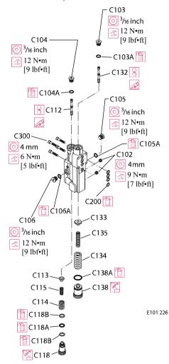
LS control shown; parts C104 through C106 and C112 through C118 are not used on PC control
