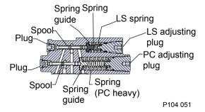
LS spool shifts to port system pressure to servo piston
