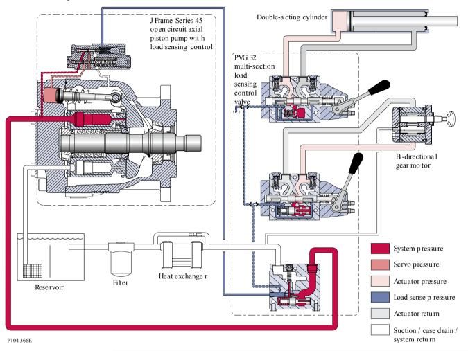
Full available flow is a function of pump displacement, operating speed, and efficiency. Refer to Series 45 Axial Piston Open Circuit Pumps Technical Information, **520L0676** for details.
