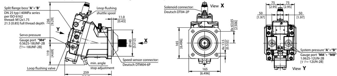
Cartridge with Electric two-position control (de-energized = min. displacement)
