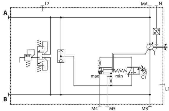
SAE ISO 3019/1 with Electric proportional control (de-energized = max. displacement)
