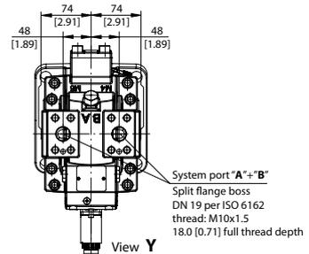
**DIN ISO 3019/2 with Electric proportional control (de-energized = min. displacement)**
