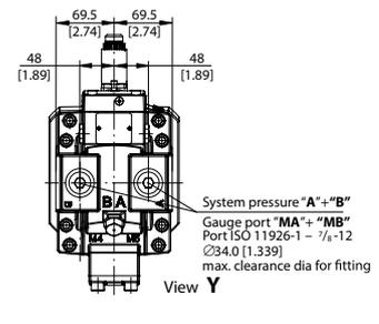
**Cartridge with Electric two-position control (de-energized = min. displacement)
