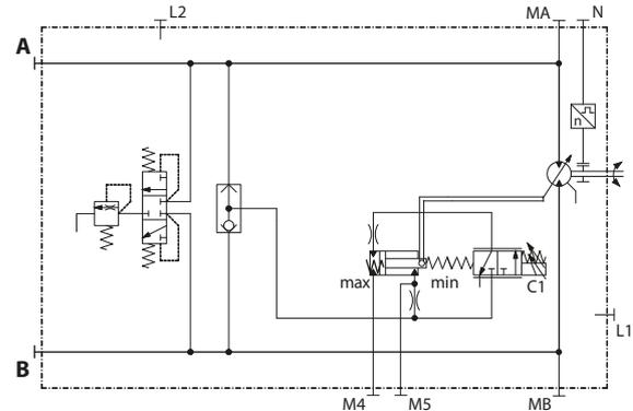
**SAE ISO 3019/1 with Electric proportional control (de-energized = max. displacement)**
