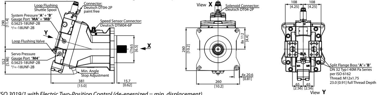
SAE ISO 3019/1 with Electric Two-Position Control (de-energized = min. displacement)
