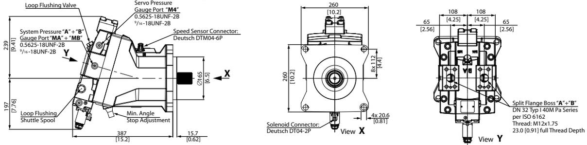
SAE ISO 3019/1 with Electric Proportional Control (de-energized = min. displacement)
