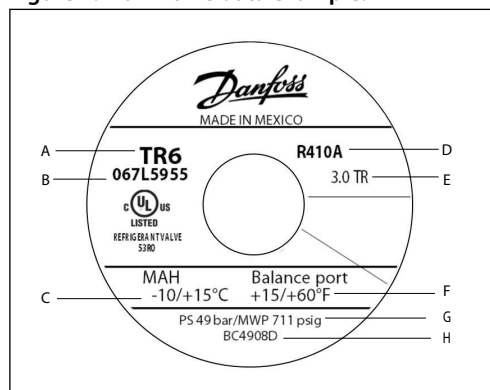
Figure 4: Main valve data example:
